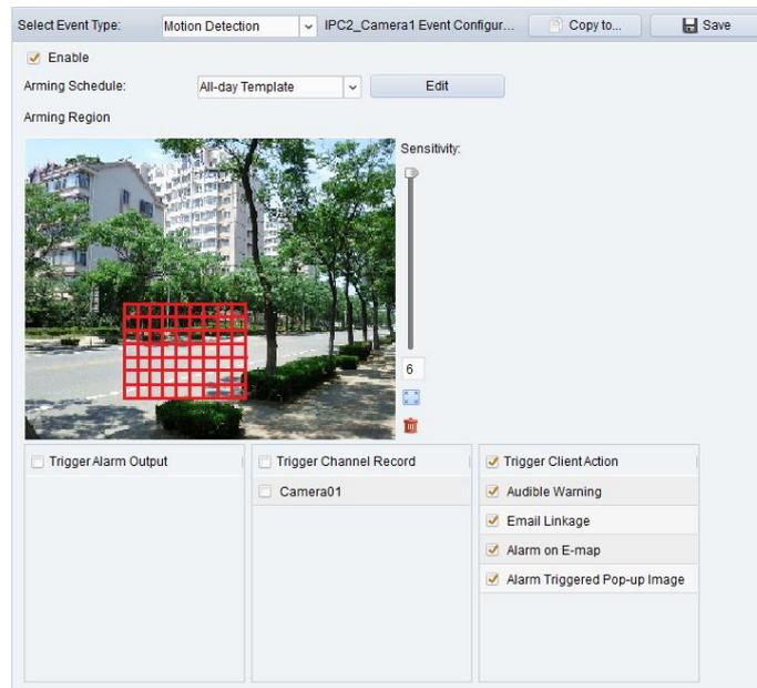
**Table 4-1 Linkage Actions for Motion Detection Alarm**
